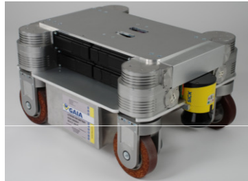
ICM-based motion controller for a pseudo-omnidirectional mobile platform
