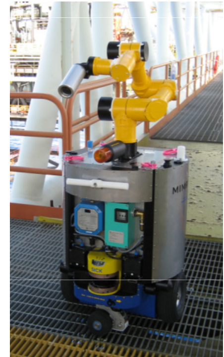
Inspection robot able to operate in explosive atmospheres
