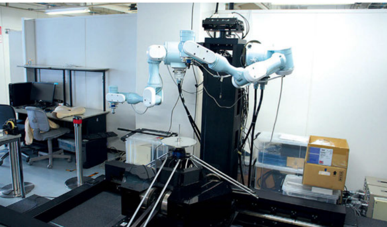
Bi-manual kinematics based on PA10 robots
